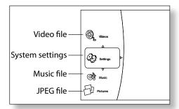
Use the (\*\*)/\*\* cursor keys on the remote control to highlight the media file type to play/view. Press (\*\*) to select the file type. The 'Play' menu is displayed:
